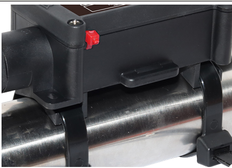
2: Two removable legs for fitting on pipes, providing a 10 mm offset from the tube. Ideal and economical for applications with low insulation thickness and pipe temperature below 100°C. Clamping on metal or PVC piping can be made by nylon tie or metal clamp (These tabs are included as standard).
